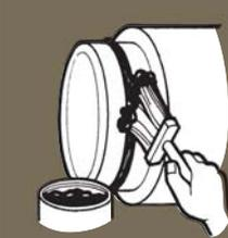
Place a clean, dry offset gasket onto a clean, dry spigot. Lubricate the gasket once it is placed on the spigot.
