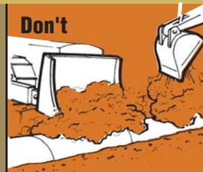
Backfill material should be readily compactible and job excavated material and should not contain large stones, boulders, frozen lumps or other objectionable material. Backfill should be placed and compacted in layers as specified.
