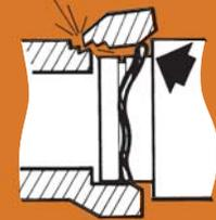
Gasket may twist out of recess, and excessive force will be required to push the pipe to the home position if lubricant is insufficient.
