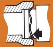
A bell not lubricated or improperly lubricated may cause gasket to roll and possibly damage the bell.
