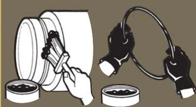
Lubricate the spigot of the pipe, including the gasket recess. Lubricate the o-ring gasket thoroughly before it is placed on the spigot or tongue.
