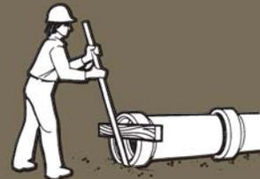
Mechanical pipe pullers or "come-along" devices are anchored to an installed pipe section several sections back and connected by a cross beam to the section to be installed. By mechanical force, the joint is brought into the home position.
