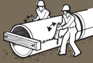
Join by placing a dead man blocking inside the installed pipe several sections back from the last installed section. This is connected to a wooden cross beam placed across the bell end of the pipe section being installed by a chain or cable and mechanical pipe puller. By mechanical force, the joint is brought into home position.
