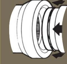
Align bell and spigot of pipes to be joined. Before homing the joint, check that the gasket is in contact with the entry taper around the entire circumference. Make sure pipe is aligned.
