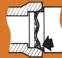
Improper alignment can dislodge gasket causing leaks or possibly break the bell.
