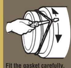
Fit the gasket carefully. Equalize the rubber gasket stretch by running a smooth, round object, inserted between gasket and spigot, around the entire circumference several times.
